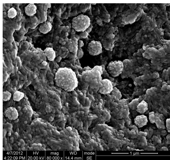
Figure 14. Secondary electron image of PC/DOP/C60 (89/10/1, wt/wt/wt) composite sample, crystallized at 300 MPa, 300°C for 9 h.
